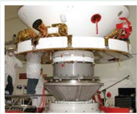
Mars Mission Satellite Testing (Photo courtesy of NASA/JPL-Caltech).
